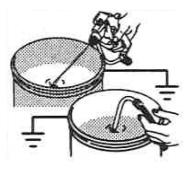
**3.** Place drain hose in paint pail. Trigger gun into waste pail and run sprayer until paint appears from gun.
