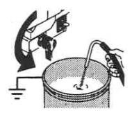
**2.** Open drain valve. Run sprayer until paint appears from drain hose. Turn off sprayer and close drain valve.
