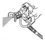
You are now ready to spray! Turn sprayer on, trigger gun and increase pressure to desired setting.
